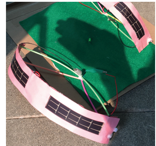
Solar modules woven into pink sail structures and illuminating green LED
